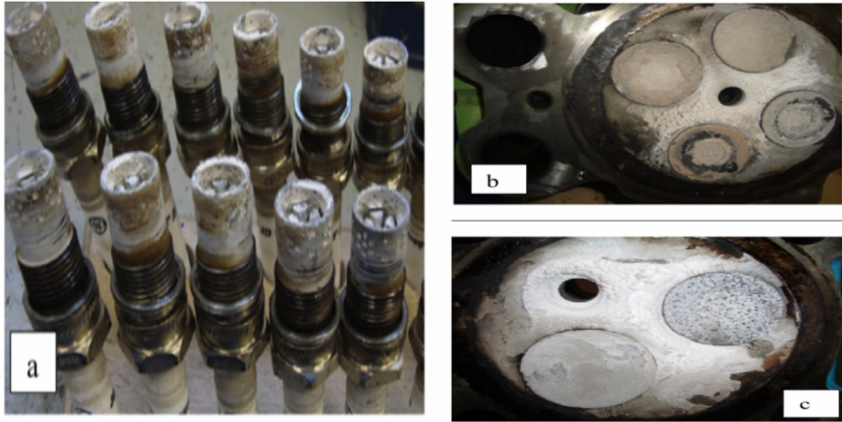
Figure 3: Examples of Equipment Damage caused by Siloxanes (a) Spark plugs, (b) engine head, (c) cylinder head.
